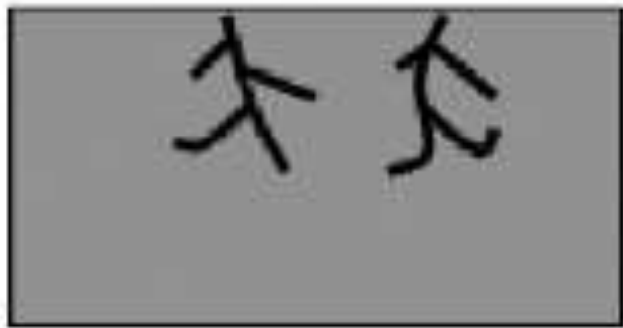
Stress corrosion cracking
