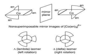
The optically active isomers of {Co(en)<sub>3</sub>}<sup>3+</sup>(top) and their directions of rotation of polarized light.
